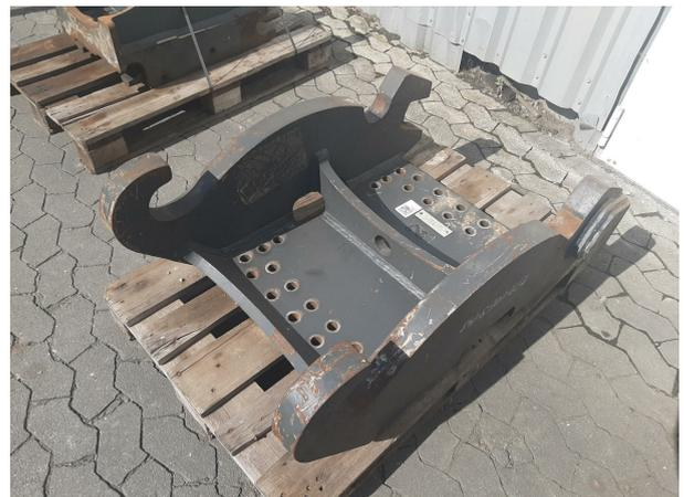
**Kaiser, Schraubadapter CW55S, Bohrbild DRP45**
